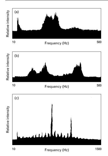
**FIGURE 3.** (a) Doppler spectrum of rainstorm echoes observed with an S-band radar. (b) Doppler spectrum of chaff echoes observed with an S-band radar. (c) Doppler spectrum of a C-45 aircraft inbound observed with an S-band radar.
