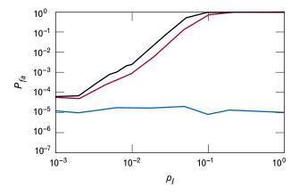
**FIGURE 4.** Probability of false alarm  $P_{fa}$  versus probability of interference  $p_{l}$ . The black curve represents data from a linear receiver with interference 100 times the noise. The red curve represents data from a linear receiver with interference 10 times the noise. The blue curve represents data from a hard-limiting receiver with interference 10 times the noise. Only the hard-limiting receiver maintains a  $P_{fa}$  value of 10<sup>-5</sup> for all values of  $p_{l}$ .
