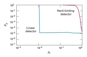
**FIGURE 5.** Probability of detection  $P_d$  at the output of a digital integrator versus the probability of interference  $p_l$ . Interference was 100 times noise. Peak signal amplitude was the square root of 10 times the wideband noise variance.
