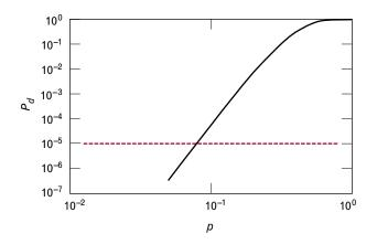
**FIGURE 2.** Probability of detection  $P_d$  at the output of a digital integrator versus the probability p of a threshold crossing on a single trial. The sliding window is sixteen units long. Eight or more threshold crossings constitute a detection. A useful detection probability of 0.9 can be attained with those values when p equals 0.625 or greater.
