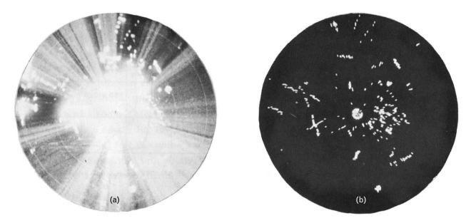
**FIGURE 6.** Comparison of displays from two receivers subjected to three jammers on a single B-47 at 35,000-ft altitude and 10-mi range: (a) time exposure of an output display of a linear receiver and (b) time exposure of the output of a hard-limiting receiver. The lines of blips represent aircraft tracks.
