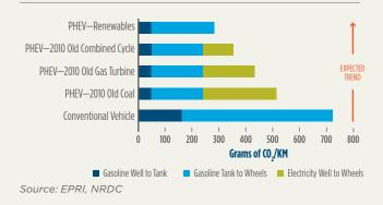
In all cases, there is an improvement in CO<sub>2</sub> emissions per mile: "well to wheel." While a PHEV that uses renewable electricity (e.g., wind or solar energy) affects a CO<sub>2</sub> reduction of two-thirds, a coal intensive power generation source reduces the well to wheel CO<sub>2</sub> emissions by one-third.
