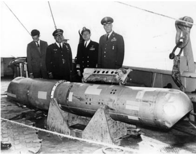
FIG. 1: The B28 warhead recovered from the ocean floor following the Palomares accident. Notice the damage to the nose caused by the impact. The underwater search effort for this weapon lasted 80 days. This image is also noted as one of the earliest publicly available photographs of a US thermonuclear weapon. Image from [12]
