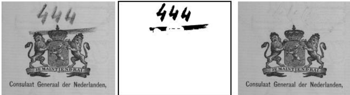
Fig.6.5: Selective removal of chalk from paper, (i) before cleaning the object, (ii) digital isolated black and white image and (iii) the after cleaning object.
