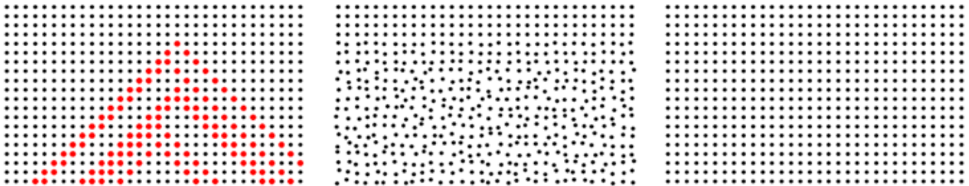
A. "As-grown" SOS with twinning defects shown in red. These defects cancel each other when they merge higher up in the silicon layer.
