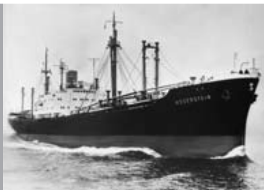
Back in familiar waters: the turbine freighter "Weserstein" from Bremen entered service in 1953 to resume the East Asia service. The freighter displaced 7,000 GRT, had 10,000 DWT and a cruising speed of 17.5 knots.
