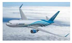
The 767-300BCF is also compatible with the winglets offered by Aviation Partners Boeing. Whether the winglets are already installed on the airplane being converted, or installed during or after conversion, the 767-300BCF operator will realize improved operational performance and reduced fuel burn relative to an airplane without the winglets.
