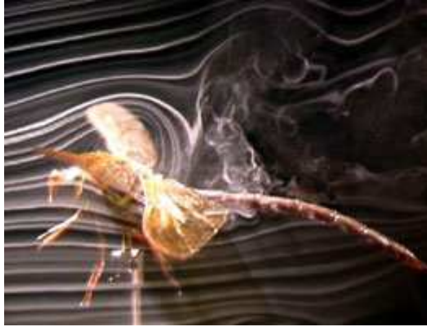
Figure 1.1: Turbulent flow created by a dragonfly (Adrian Thomas, Dept. Zoology, Oxford University)
