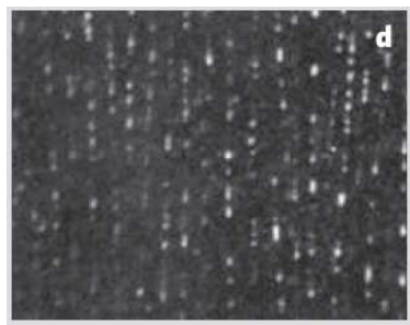
Figure 7.5: Micron-size solid hydrogen particles trapped in a vortex lattice in superfluid helium, as observed by Bewley et al. (2006).
