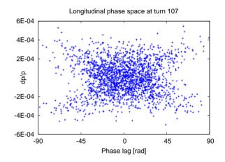
Figure 4: Longitudinal phase space plot at the end of the capture process with 202 MHz, with a 300 ns long barrier bucket. A starting dp/p = $7 \times 10^{-5}$  was assumed. This is a simulation result including longitudinal space charge forces.
