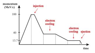
Figure 6: Schematic view of ELENA cycle.
