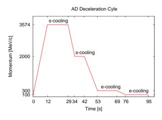
Figure 1: The AD deceleration cycle.
