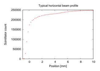
Figure 2: A typical horizontal beam profile obtained by the scraper at 100 MeV/c. The  $\beta_h = 5m$  at the scraper position,  $\epsilon_h = 0.5 \pi$  mm mrad with 80 % of the beam inside and with a long tail of the distribution.
