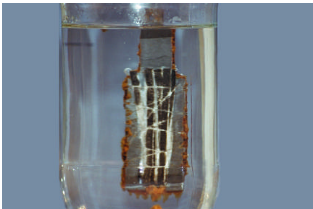
Figure 4. Close-up of the magnesium protected sample
