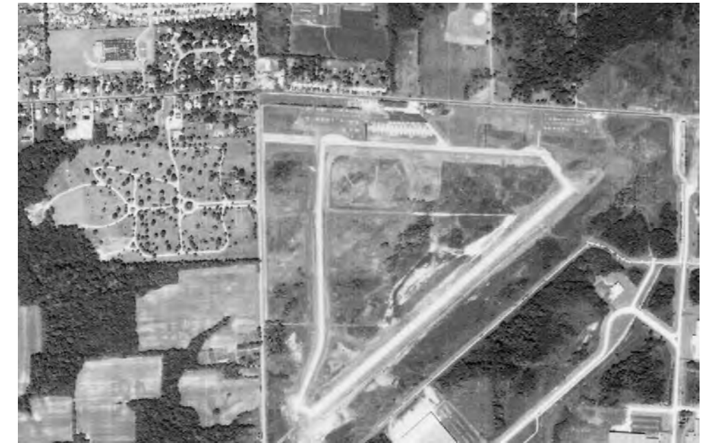
By 1977, the Airport’s original grass runways were abandoned and a new paved runway and taxiways were installed where they remain today. 1977 aerial photo provided by Environmental Data Resources.
