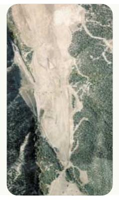
Phase I bond release was granted following backfilling and grading of the mine site and drainage reestablishment. Topsoiling and revegetation are in process.
