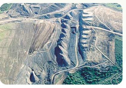
Left: Inspections include sampling for vegetative cover. Above: This photo shows the stages of mining and reclamation in a surface coal mine. From left to right: revegetation after two growing seasons; revegetation after one growing season; replaced topsoil; regraded spoil; spoil ridge; open pit; disturbed lands where topsoil has been salvaged. Right: Sampling mine discharge is often part of the monthly inspection routine.
