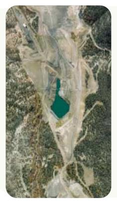
Phased reclamation of the Tomahawk Strip Mine in Delta County. This photo shows the early stages of reclamation grading.
