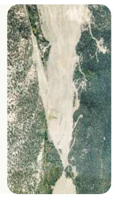
Phase II bond release was approved after topsoil was replaced and vegetation was established to control erosion and support the post mining land use.
