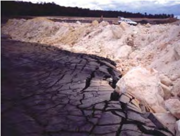
Waste rock pushed into desiccated tailings
