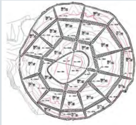
Plan showing surface cells to capture rainfall and to minimise erosion on slopes
