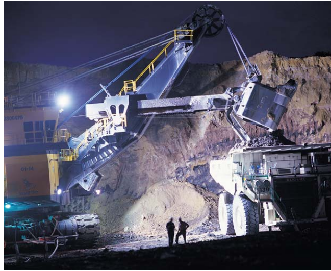
Figure 4.4: Overburden loading by electric shovel Photograph courtesy of Premier Coal
