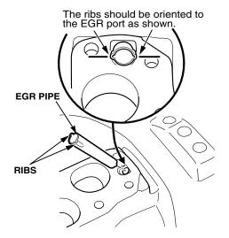
13. Use the installation tool and a small hammer to drive the EGR pipe into the port until it is flush with the port. Make sure the pipe will not contact the gasket after installation.
