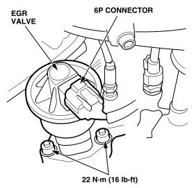
17. Install the new EGR valve with a new gasket. Torque the mounting nuts to 22 N·m (16 lb-ft). Reconnect the 6P connector.  Install the intake manifold with the original gasket. Torque the mounting nuts and bolts to 22 N·m (16 lb-ft) sequentially in two or three steps. Route the PCV hose so it is not pinched under the intake manifold.
