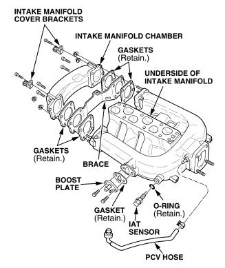
6. Cover the six ports on the bottom of the manifold with duct tape.
