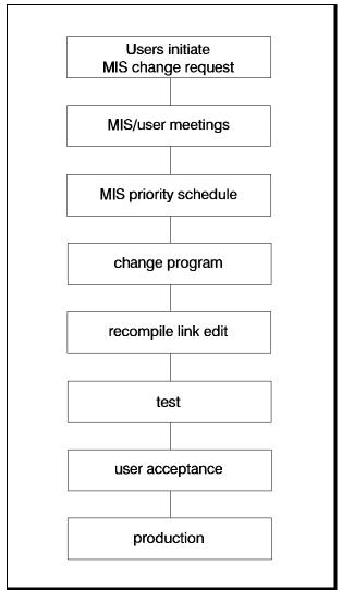
Figure 2 lists the steps in processing a typical change request for a traditional procedural application.
