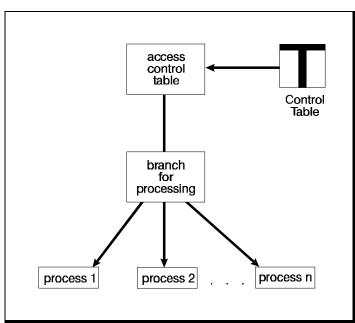
Figure 7 Using Control Tables to Drive Program Logic
