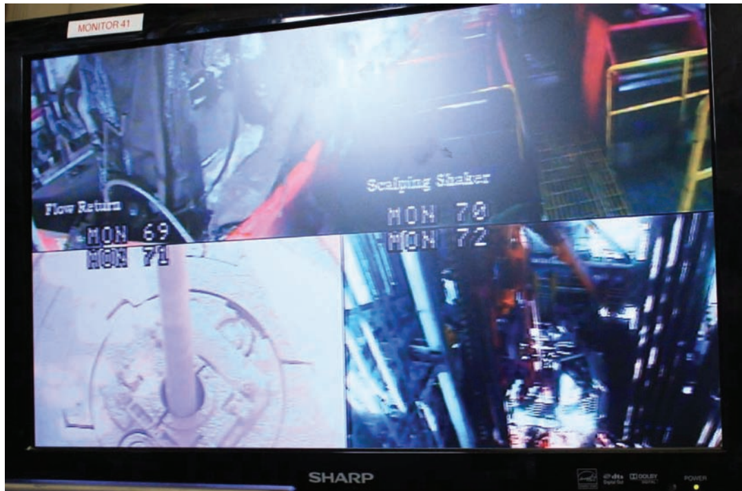
Figure 12. Typical Video Camera Displays in the Driller's Cabin (not Deepwater Horizon ).
