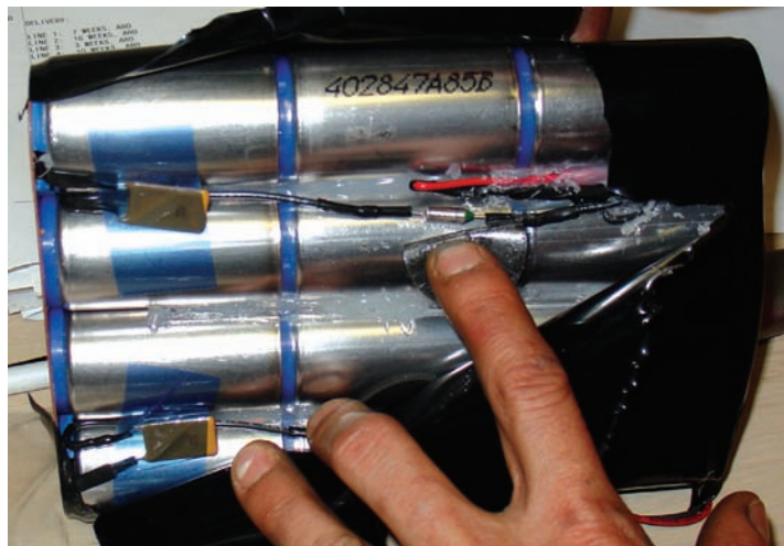
Figure 17. Photograph of a 9-volt AMF Battery Pack. (Not from Deepwater Horizon BOP pod.)
