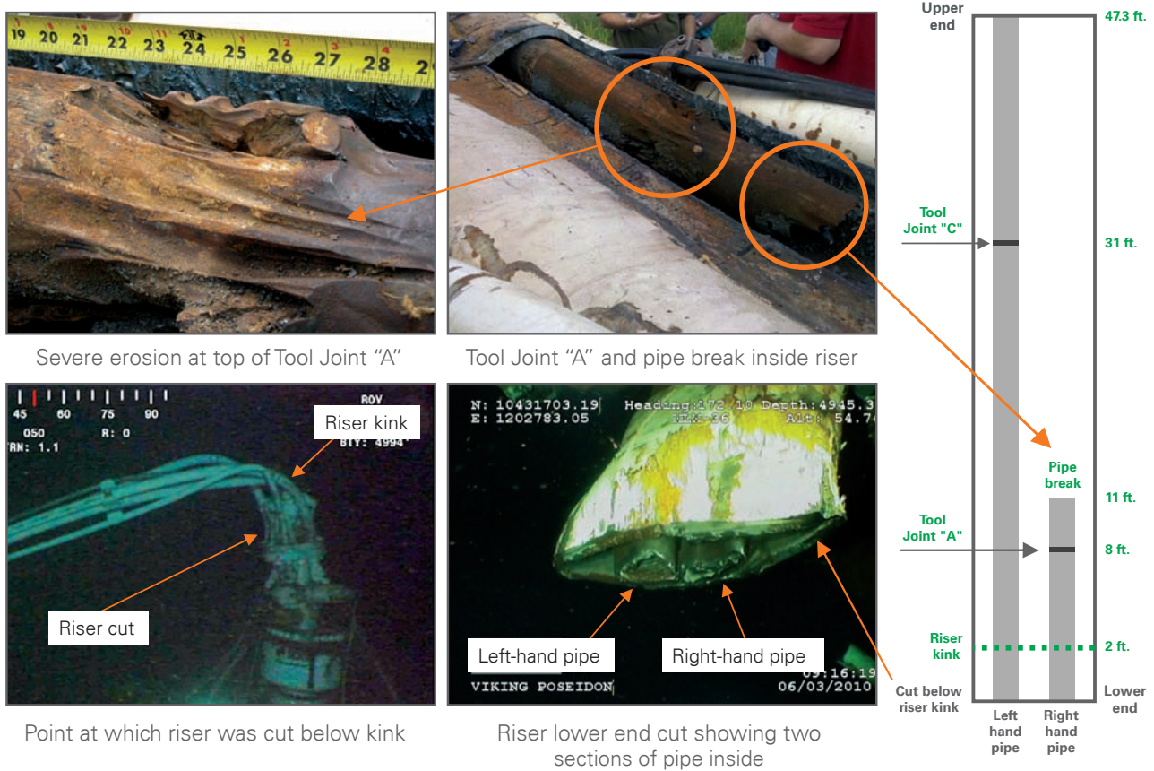
Figure 14. Retrieved Riser Kink Section and Its Contents.
