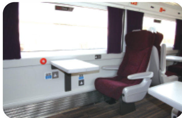
New Wheelchair Space with Call for Aid and Power Sockets
