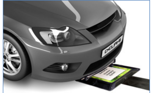
The Delphi Wireless Charging System eliminates the need for a charging cord. Drivers can park their electric vehicle over a wireless energy source that sits on the garage floor or is embedded in a paved parking spot.
