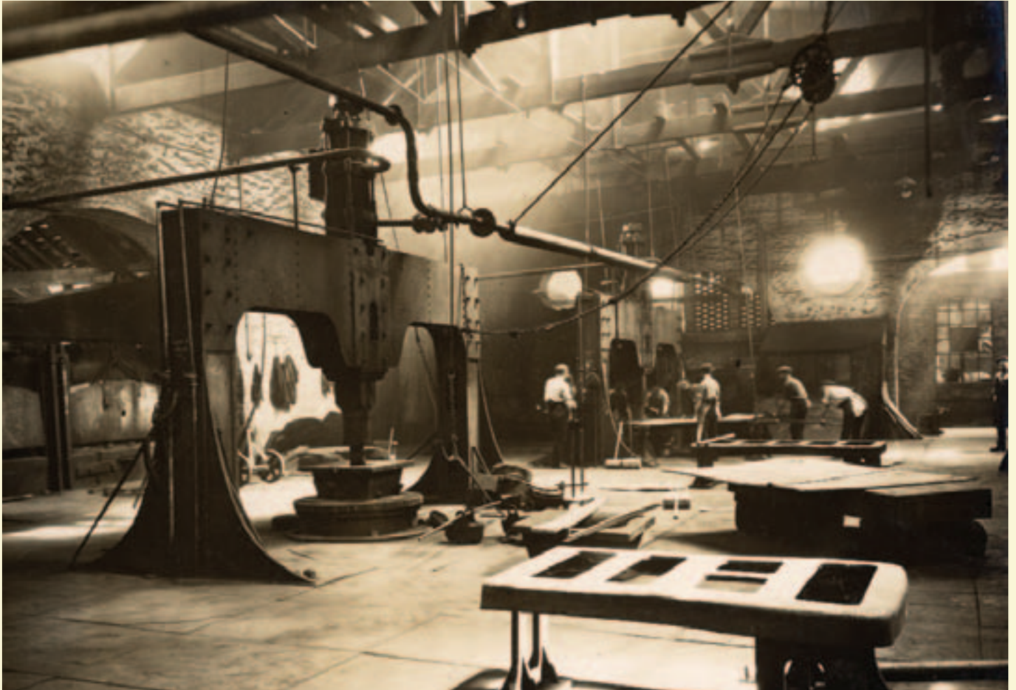
Hafod Copperworks interior showing a steam hammer used for hammering copper plates
