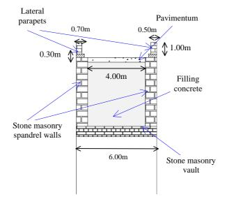
Figure 2: Bridge cross section
