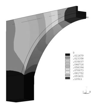
Figure 7: Displacement field [m]
