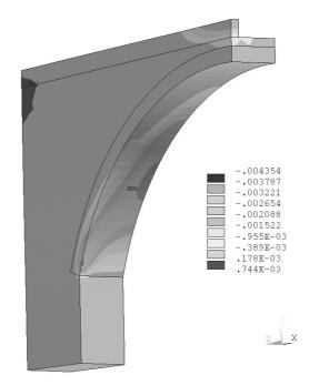
Figure 5: Strain distribution [m/m]
