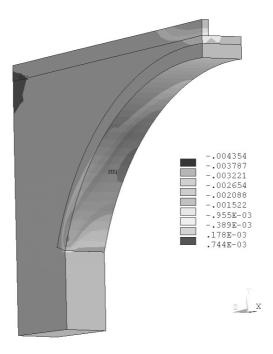
Figure 6: Maximum plastic principal strain [m/m]
