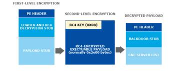
*Figure 2. File structure of encrypted SIMBOT malware variants*
