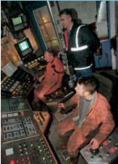
Doghouse on Galaxy-1 drilling rig.
