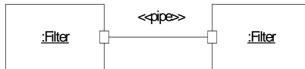
Figure 17: A C&C Connector as a UML Association (Link)
