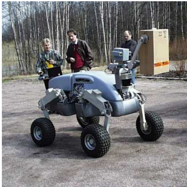
Figure 1.15: The WorkPartner robot, with hybrid wheel-leg locomotion system.
