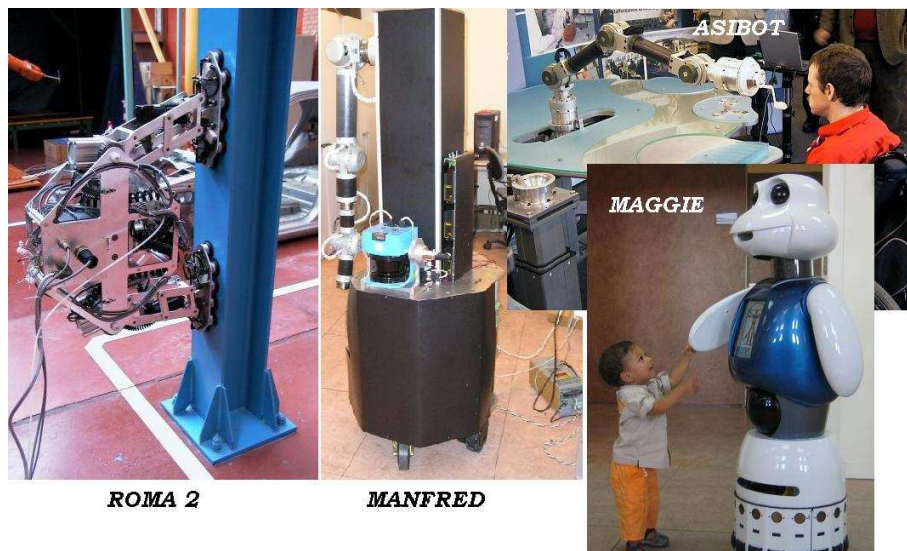
Figure 1.5: Examples of services robots. University Carlos III of Madrid, some Roboticslab service robots: ROMA 2 (climbing robot for inspection), Manfred (mobile manipulator), ASIBOT (Portable assistive robot), Maggie (Personal social robot).
