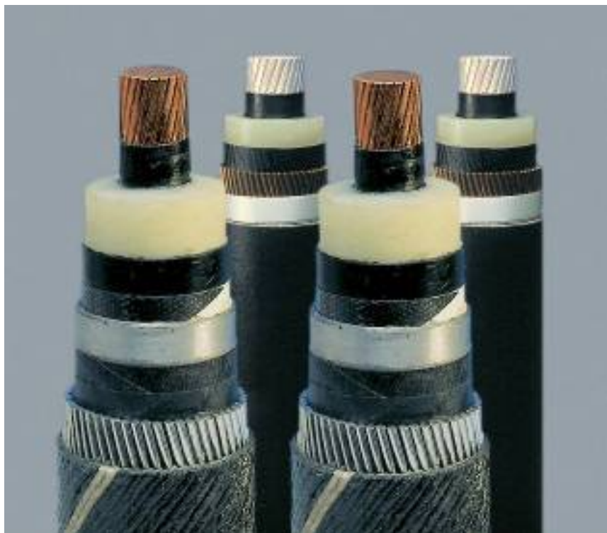
Fig 1. Polymer insulated cables. Submarine cables in front and land cables at the rear
