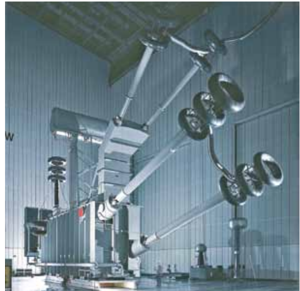
Fig. 5.2-1: Converter transformer for the Tian Guang HVDC project during type test
