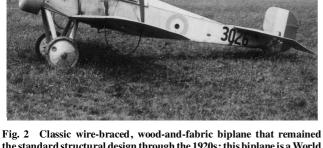
Fig. 2 Classic wire-braced, wood-and-fabric biplane that remained the standard structural design through the 1920s; this biplane is a World War I Bristol Scout (SI negative number 78-18721).
