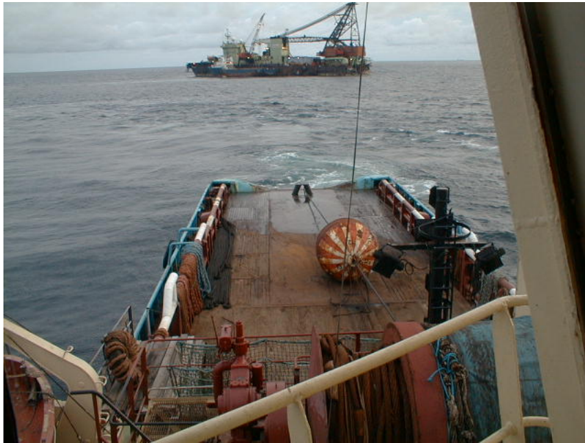
Photo showing pennant wire going through the buoy on aft deck.
