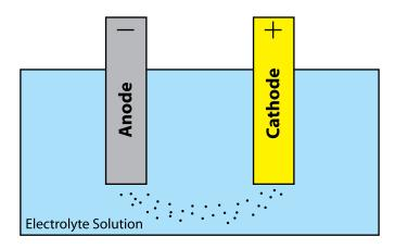
When the two dissimilar metals come into contact, the electrical loop is closed, and the natural voltage differential between them causes electron flow. One metal will become the anode (negative) and one will become the cathode (positive).
