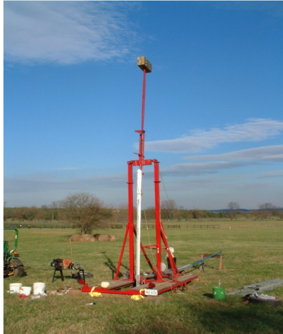
A King Arthur style trebuchet in the cocked position. This design, while producing the best results today, would not scale down well (FAKA).
