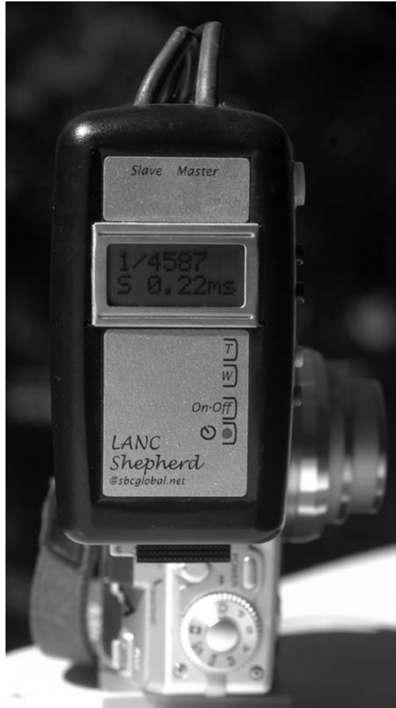
FIGURE 4.6 The LANC Shepherd remote controller for stereo cameras.
