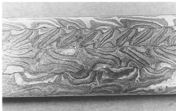
Figure 14. Detail of blade on a peidao , 17th–18th century, showing four-row huawengang and inserted edge plate. Courtesy Scott M. Rodell, Great River Taoist Center, Washington, D.C. (photo: author)
