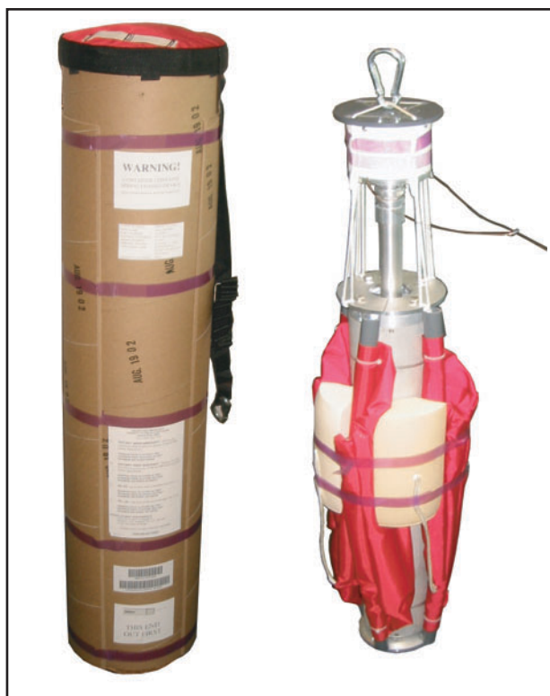
Figure 4. Left: A METOCEAN SLDMB deployment packaging tube. Right: An SLDMB removed from the tube.
