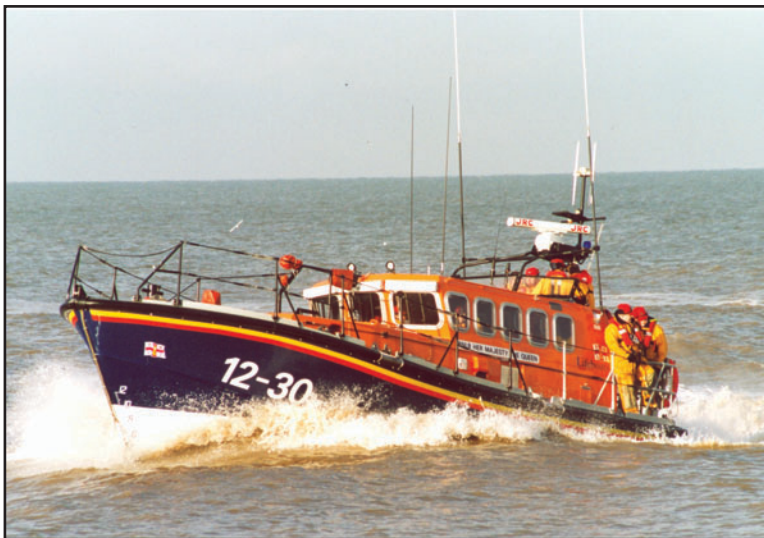
The 38-foot Mersey class RNLI carriage-launched lifeboat. This vessel is one of five current classes of all weather lifeboats, ranging from 38- to 55-feet.
