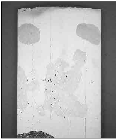
Fig. 3b. Area on working surface of inner liner where EBC appeared to be intact or only slightly damaged.
