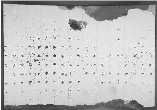
Fig. 3c. "Pinhole" pattern observed on working surface of outer liner.
