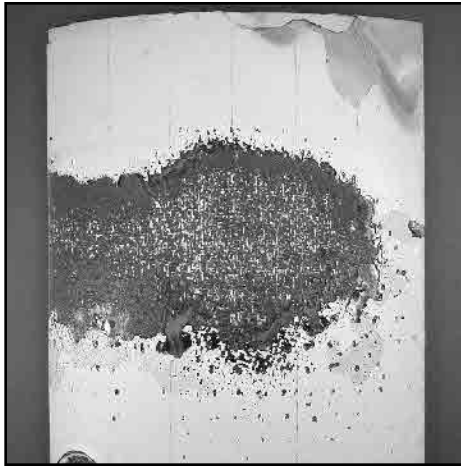
Fig. 3a. Severely damaged area on working surface of inner liner corresponding to a typical fuel injector impingement area.
