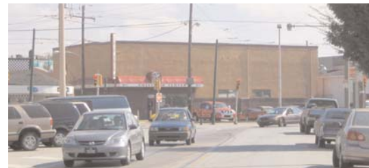
Reed Street (foreground) abruptly changes its direction at Passyunk Avenue. The existing CVS parking lot (beyond) has no visual buffer. The street and the surface parking lot blend into a confused auto-oriented environment. A low brick wall with iron pickets would screen headlights of cars within the parking lot and provide an appropriate termination of this view.
