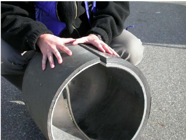
Wall thickness comparison - 35 MPa vs 70 MPa cylinders
