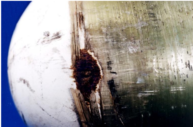
Tank dragged on road under vehicle after support strap broke.
