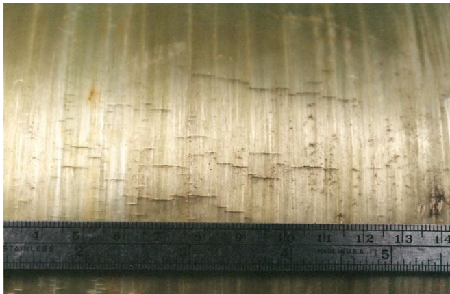
Stress corrosion cracking due to acid attack on fibers
