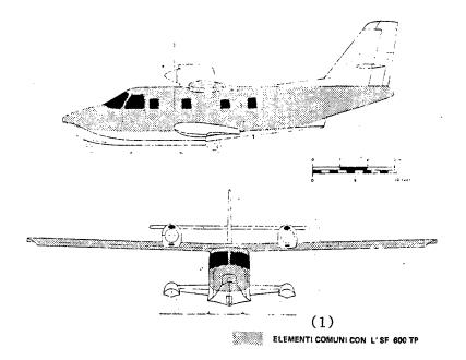
In this drawing, the elements that are common with the SF-600TP are shaded. Key: 1. Elements common with the SF-600TP
