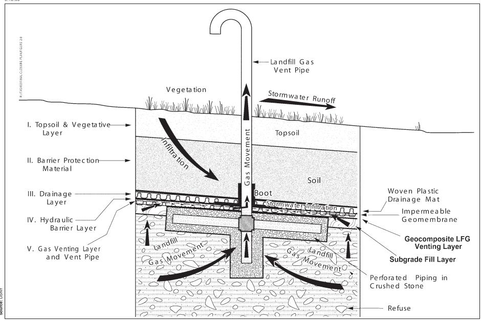
Final Cover and Landfill Gas Venting System Landfill Sections 1/9 and 6/7
