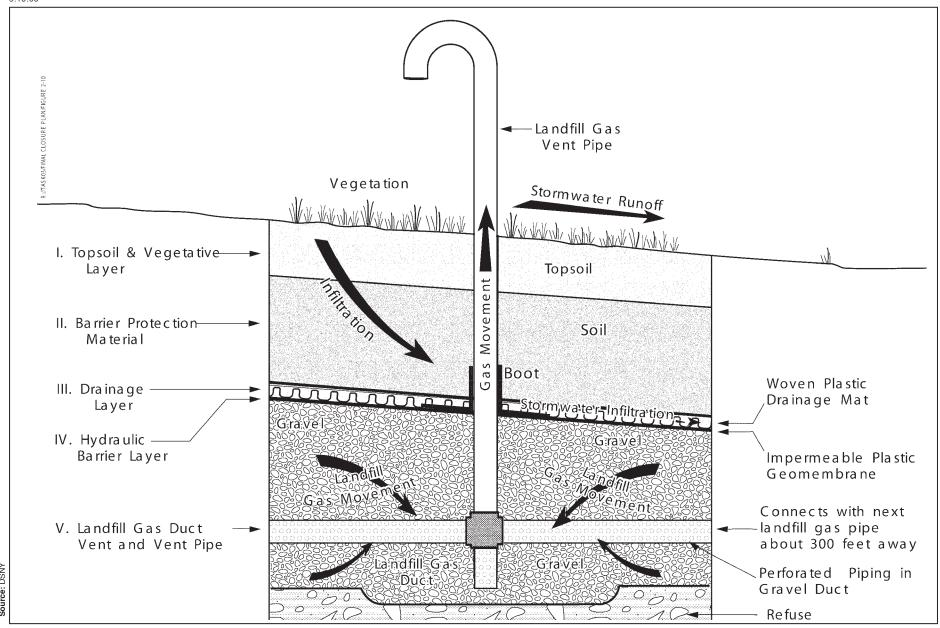
Final Cover and Landfill Gas Venting System: Landfill Sections 2/8 and 3/4
