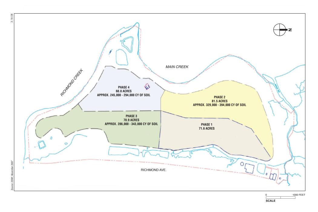
Final Closure Construction Phasing for Section 6/7
