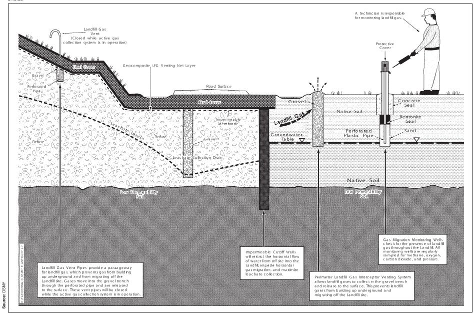
Cross-Section of the Landfill Gas Venting System
