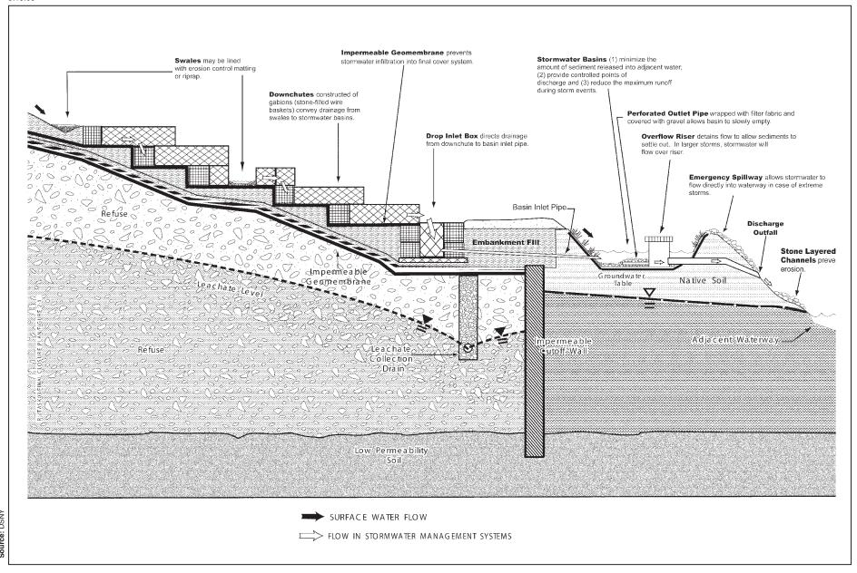
Cross-Section of the Landfill Drainage System Landfill Sections 1/9 and 6/7
