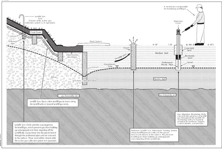
Cross-Section of the Landfill Gas Venting System Landfill Sections 2/8 and 3/4
