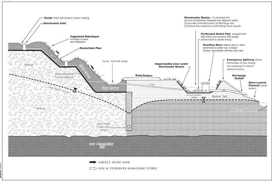
Cross-Section of the Landfill Drainage System Landfill Sections 2/8 and 3/4
