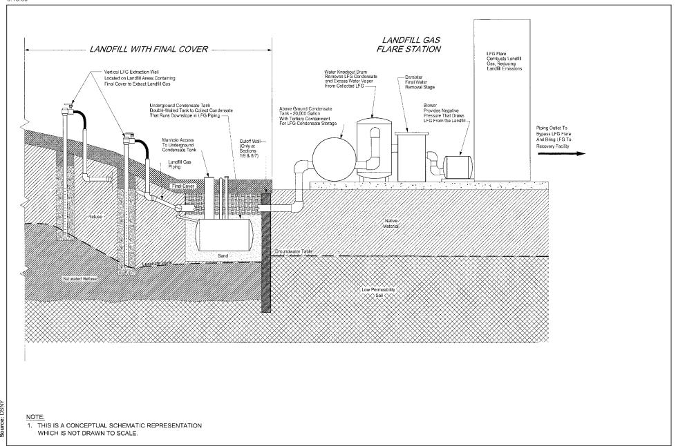
Active Landfill Gas (LFG) Collection System Figure 1-8a
