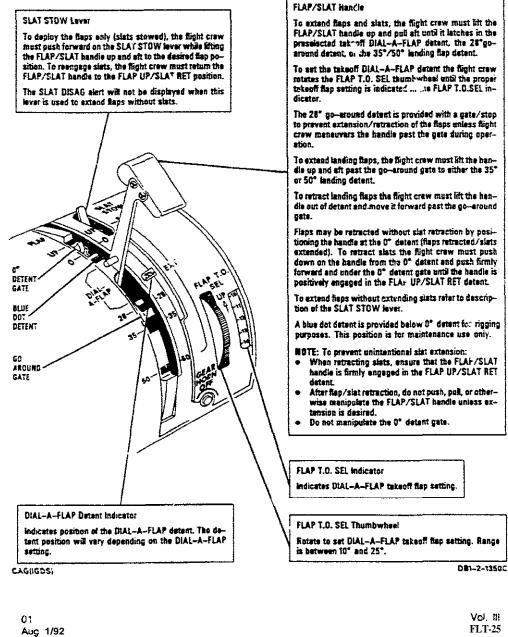
Figure 4.--Flap/slat handle module.
