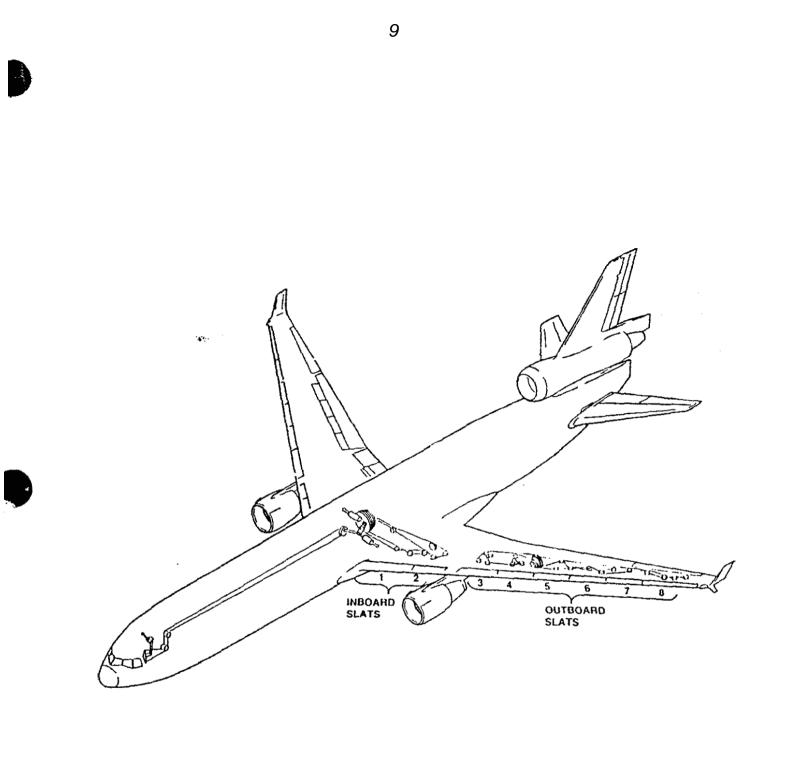
Figure 1.--Slat cable system.
