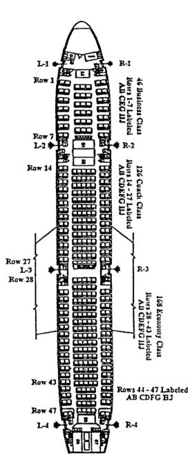
Figure 6.--Passenger cabin configuration.
