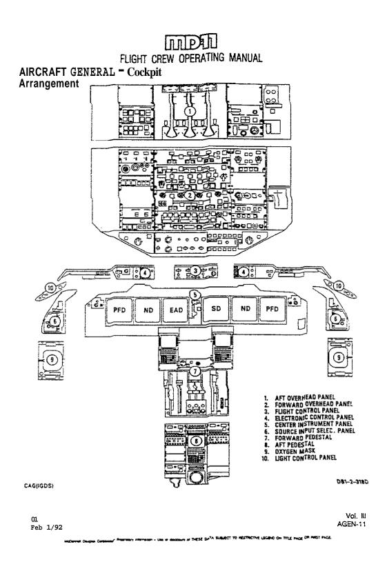
Figure 2.--MD-11 cockpit arrangement.
