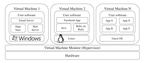
**FIGURE 1.2.** A hardware virtualized server hosting three virtual machines, each one running distinct operating system and user level software stack.
