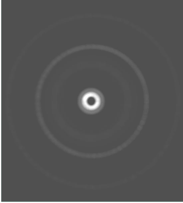
Figure 2.7: Hg Pen Lamp Emission: Output of CTEEx Through 360° Rotation of the Prism[4]
