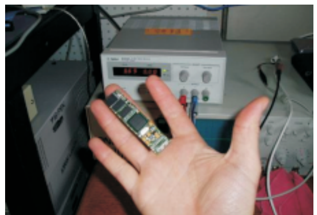
Gumstix single-board computer is as small as a gum stick
