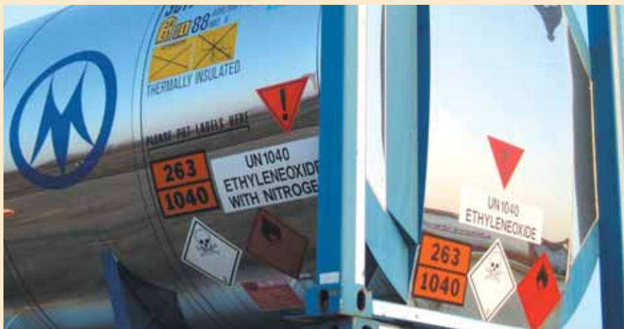
Figure 5: Dangerous goods label and hazard identification number
