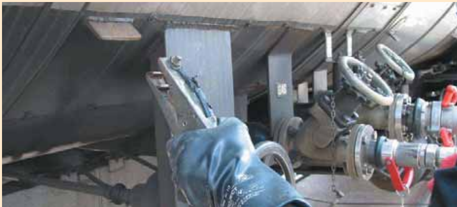
Figure 2: earthing connection of a Railway Tank Car
