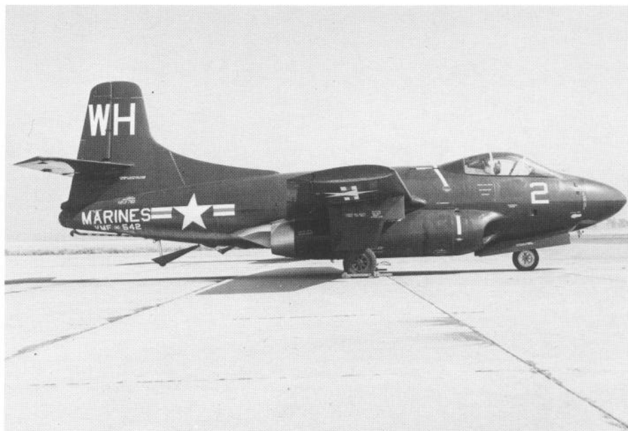
Top right, rearmed aircraft being positioned for takeoff at K-3 Korea. Right, the first night jet kill was accomplished with a Douglas F3D Skyknight.
