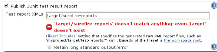
Figure 6.10: Configuring the JUnit test result report post build action
