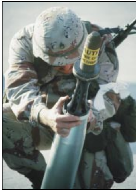
DoD file photo An ammunition specialist examines a 105mm armor-piercing, discarding sabot round, to be used in an M-1 Abrams main battle tank, during Operation Desert Shield.
