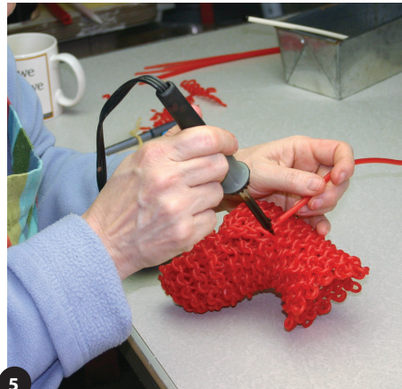
5 A complex set of "sprues," "gates," and "vents" are soldered to the piece with wax to provide pathways for glass to enter and air to leave the piece. Photo: Steve Isaacson.
