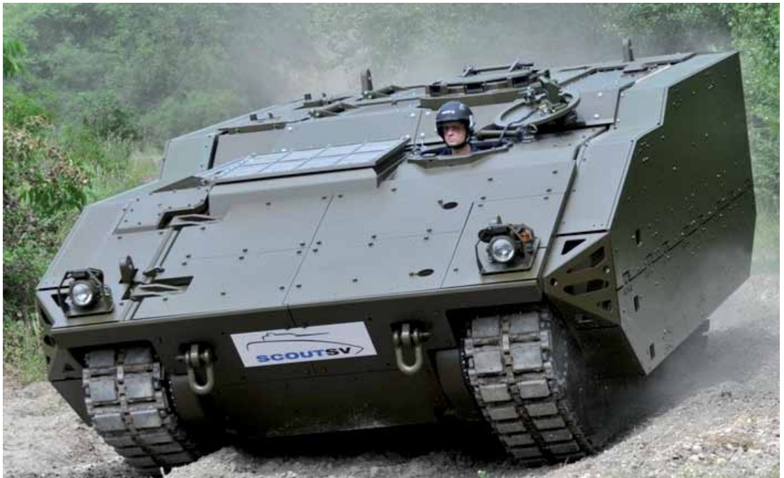
The Scout Specialist Vehicle Mobile Test Rig has been rolled out at a General Dynamics facility in Vienna, Austria. The vehicle is seen here with the additional armour pack for Theatre Entry Standard levels of ballistic protection
