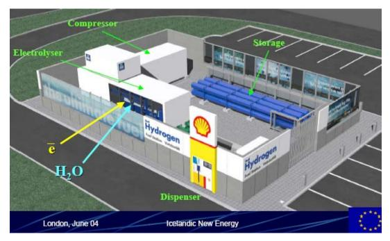
Figure 2: The Icelandic hydrogen refueling station
